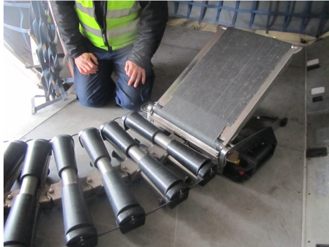
Figure 6 shows the extended arm and elevated lip on the Power stow.
