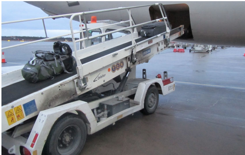
Figure 8 shows a regular loading belt being used when loading
