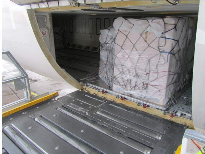
Figure 4 shows cargo that has been rolled into the cargo compartment by the high loader.
